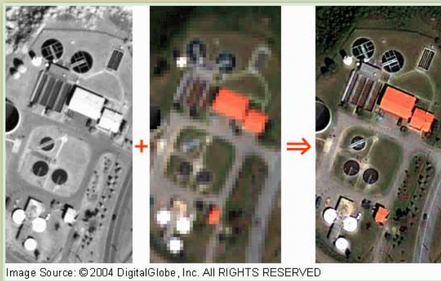
Figure 9: Pan-sharpening process by fusing panchromatic and multispectral image
